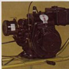
Tecumseh 4-cycle engine—with easy-pull recoil starter, float type carburetor and mechanical governor that makes additional power available as load requirements vary. Special mini-bike control adapts carburetor to remote handlebar operation.
