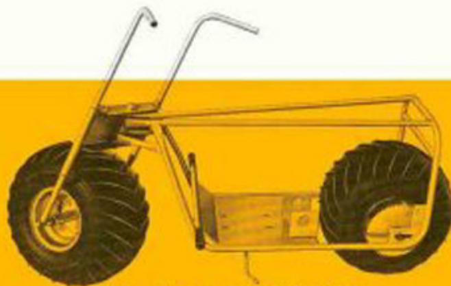
Shows the assembly of the front fork and wheels.
