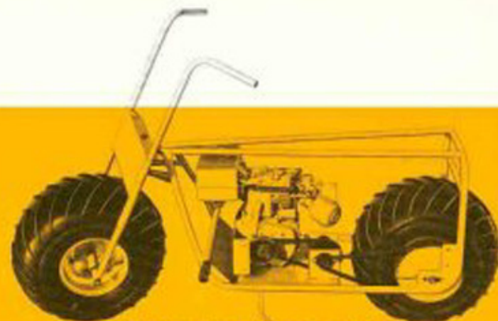
The engine, clutch and drive chains in position.
