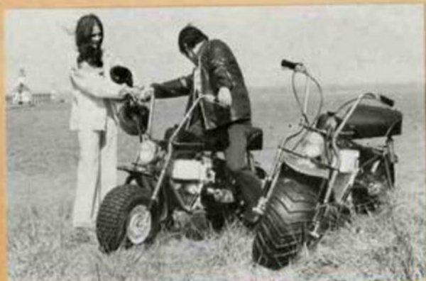
The only difference between VT-8 and -812 is front fork and tire.
