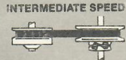
C. As engine goes faster, clutch continues to close. Belt forces driven pulley wider. Drive ratio is about 10:1.
