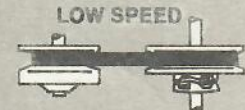
B. As engine speeds up, clutch closes forcing belt up beveled sides. Belt tightens and begins turning driven pulley. Ratio is for power (approx. 18:1) to get going.
