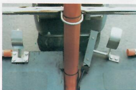
You can get foot controls on your Super Tryke with optional bench seat. Accelerate and brake just like a car. Special modifications available to accommodate physical handicappers - just ask for details.
