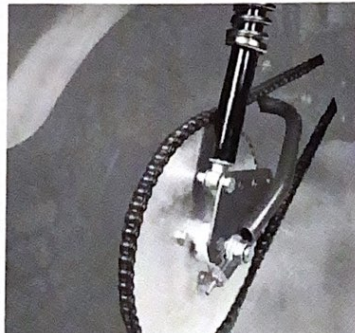
Chain and sprocket assembly can be adjusted by loosening one nut.
