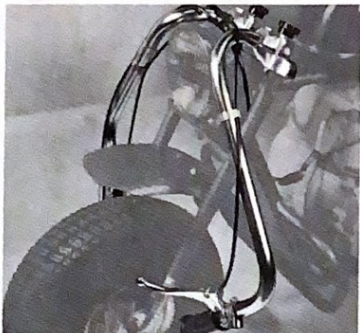
Handlebars fold down for maximum portability, quick and easy storage.
