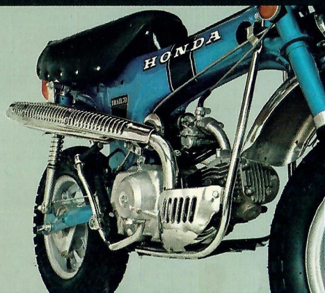
The 70 features a sweptback, covered tailpipe and a dependable four-stroke 5 hp engine.
