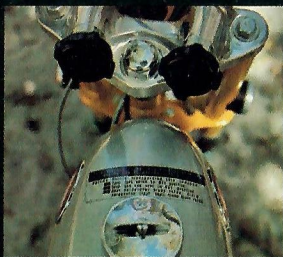
Safety lock gas cap and turn-lock knobs for the fold-down handle bars.
