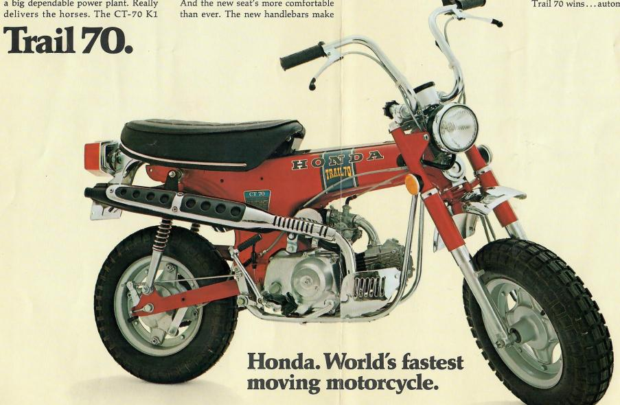
Transmission . . . . . . . . . 3 speed, with automatic clutch.
