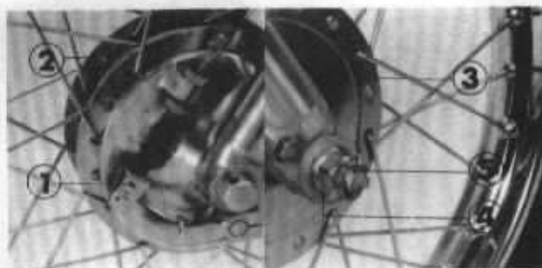
Fig. 4-2 1. Cotter pin 2. Front brake cable 3. Cotter pin 4. Front axle nut 5. Front axle
