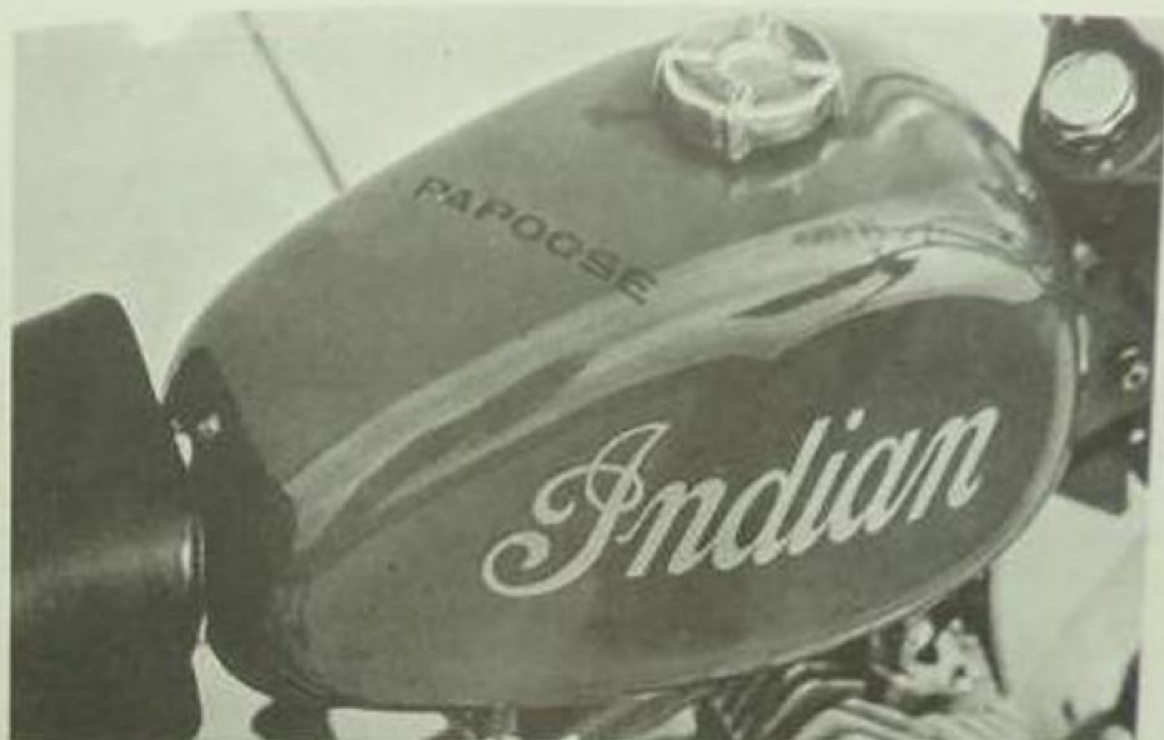
The gas tank holds just over a gallon — enough for a hundred miles riding
