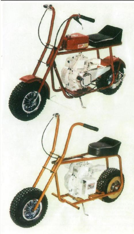
RUPP C-250; 21/2 HP Tocumseh engine • single speed automatic clutch • painted fenders • chrome chain guard • chrome wheel rims • naugahyde upholstery • telescoping spring loaded suspension front • twin frame construction • retractable foot pads • kickstand • rear disc brake • plastic motorcycle grips • sealed ball bearings • kandy red color
