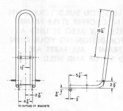
BUILD YOUR OWN HEAVY DUTY SEAT FRAME/SISSY BAR. THIS IS THE SAME ONE THAT IS FOUND ON ALL RUTTMAN CHOPPERS. THIS KIT USES RUTTMAN CHOPPER SEAT NO. RC179 BUT MAY BE ALTERED TO TAKE A DIFFERENT SEAT OR ADAPTED TO FIT OTHER MINI-BIKES.
