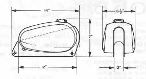
This unit, complete with automotive type twist cap, has the most recent "sculptured" look. Its overall teardrop shape is 12" long, just enough to fit many popular mini-bikes. It is baffled in its design and has ample mounting facilities. It will hold 4 1/2 quarts, plenty for miles and miles of riding.
