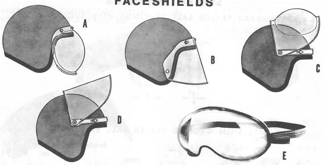
SNAP-ON BUBBLE SHIELD cuts drag and turbulence to reduce rider fatigue. Dual snaps permit use with or without a separate sun visor.
