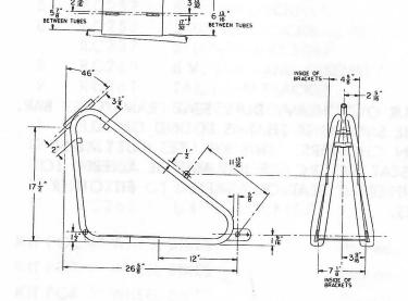
THIS KIT LETS YOU BUILD YOUR OWN RUTTMAN CHOPPER STYLE FRAME. THESE PARTS MAY ALSO BE USED AS A BASIS FOR DESIGNING YOUR OWN CUSTOM FRAME. ALL PARTS ARE READY TO SET UP AND WELD.
