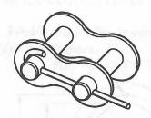
Positive locking link for high speed or racing.
