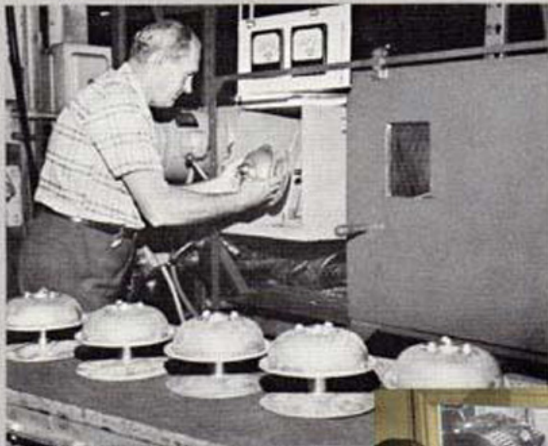
Production test of Salsbury converter driver pulley.
