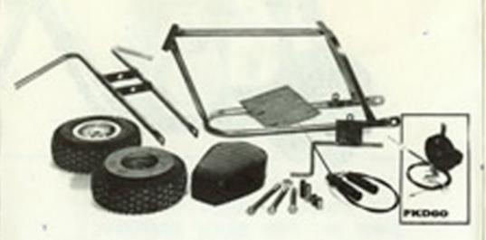
Pre-welded frame, forks. You weld engine mount to fit your engine. Includes tires and tubes, 5-in. wheels, 70T sprocket, twist throttle, friction brake, saddle. Complete except engine, clutch, chain.
